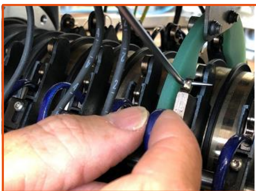
Tool for lifting the spring and checking the condition of the brush
