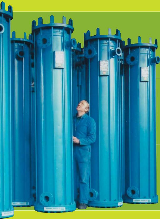
**1 -CL Clad®** makes it possible to produce high-performance anticorrosion equipment, especially distillation columns and reactors used in the fine chemicals and pharmaceuticals industries.
